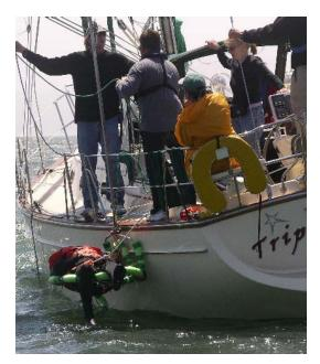
*The Lifescoop*, a full-size stainless steel stretcher with a long handle, was designed to retrieve a victim at a short distance from the boat without having to put another person in the water. Using the handle, the crew on deck maneuvers the stretcher out from the boat and under the victim, pulls it and the victim to the boat, and hoists them on deck with the jib sheet and a tackle suspended from the boom.
