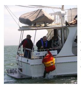
Collapsible fabric ladders and other "soft" ladder-like devices are appealing, in part because they often have an arrangement of Velcro and a trip line that allows them to be deployed by a swimmer. Stiff fingers and feet did not always feel secure on the typical small rungs, however, and the bottom rung and legs often slid under round-bottom hulls.
